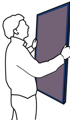
2. Place top of mirror frame over top tabs of H bracket
