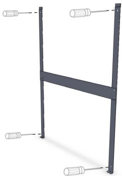
1. Screw H bracket to wall
