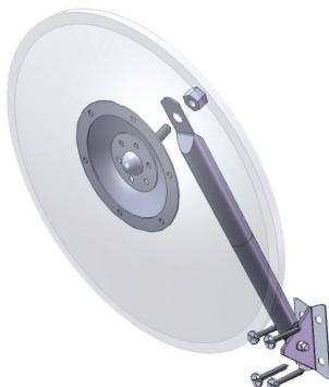
**3** Back off 1 or 2 screws on hub, 1/2 turn only. Adjust angle of mirror, retighten hub screws.
