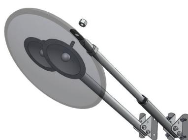
**3** Back off 1 or 2 screws on hub, 1/2 turn only. Adjust angle of mirror, retighten hub screws.
